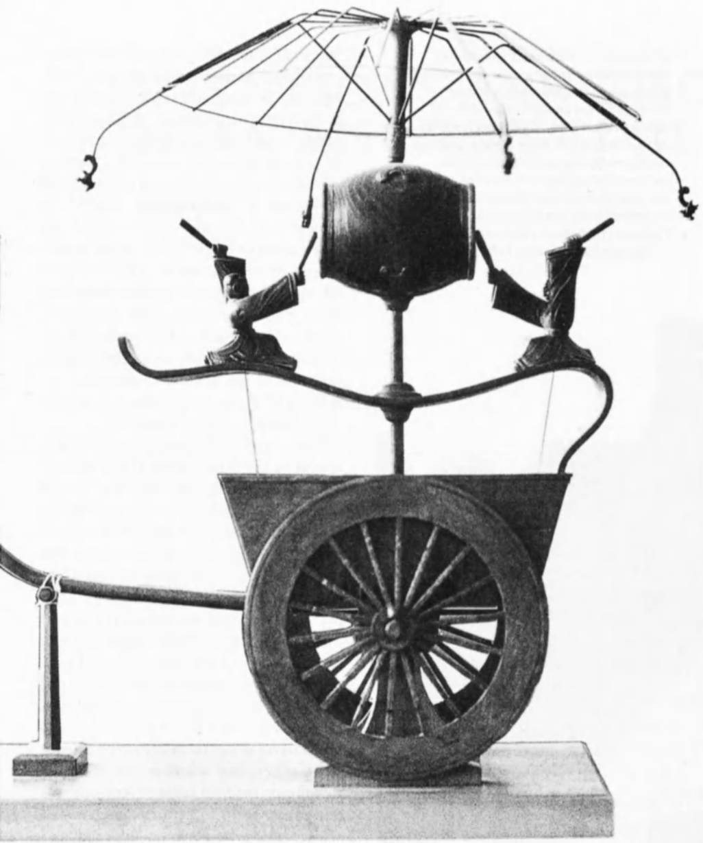
Left, a model reconstructed after a Tang Dynasty (7th century) original, of a "li-counter" or device for measuring distance. The counter was constructed in such a way that, as it moved along the road, one of the 2 drummers would beat the drum at each li , an ancient Chinese distance unit corresponding to half a kilometre.
