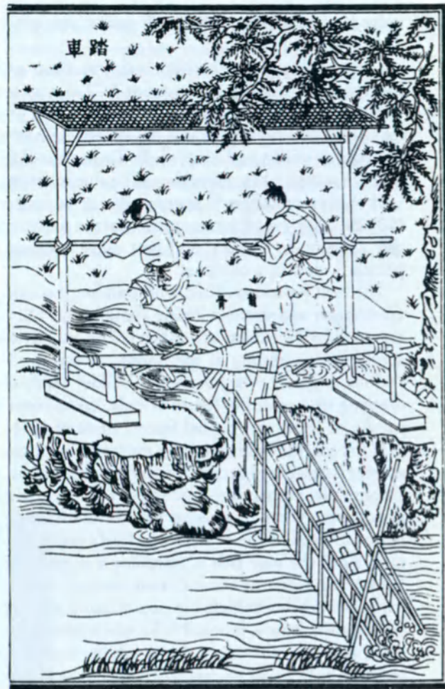
Raising water for irrigation in 17th-century China, using a two-man treadle-operated chain pump.
